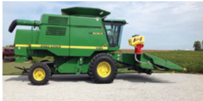
In addition to the air seeder attached to the corn head, a stalk devastator attachment is shown. The cover photo on this guide was seeded using this method.
