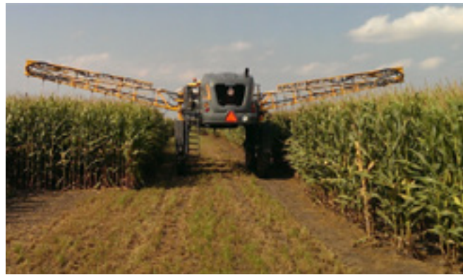
High clearance sprayer with air seeder attachment. Drop tubes place the seed under the upper canopy. This works for both 30" corn and soybean rows with very little crop damage.
