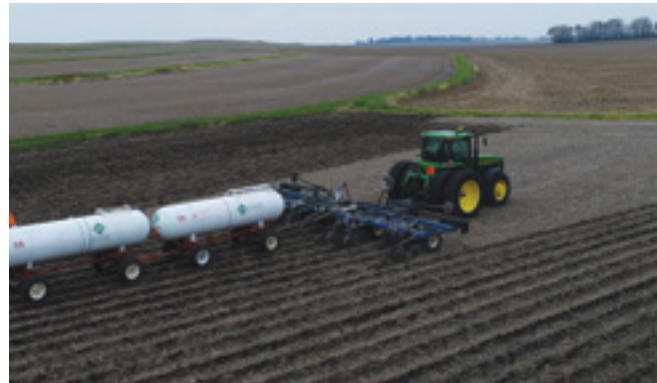
Fall anhydrous ammonia application using guidance to provide strips for planting in the spring. In the spring, use of a strip freshener with RTK guidance is recommended.
