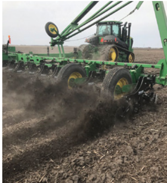
Strip freshener used on fall anhydrous ammonia applicator strips prior to spring corn planting. This was the only tillage pass and needs precision guidance such as RTK.
